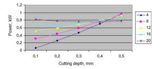
**Fig. 2.** Variation of power consumption during the sanding of black alder wood at an angle of 45 degree to the grain orientation when using the sequence of 120 grit size as a function of feed speed and cutting depth
