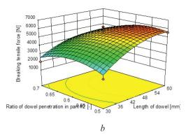
**Fig. 3.** Response surface plot showing the effect of ratio of dowel penetration in the main part of joint and the length of dowel on the breaking compressive force (a) and breaking tensile force (b). The distance between dowels was considered equal to 32 mm
