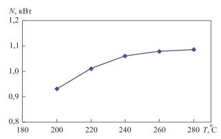
Fig. 3. The dependence of the power of engine from the temperature of torrefaction of biomass fuels
