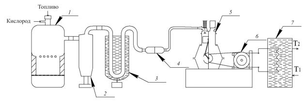
Fig. 1. The scheme of a technological complex for development of electric energy: 1 — gas generator; 2 — cyclone for gas cooling; 3 — coiled heat exchanger; 4 — filter; 5 — internal combustion engine; 6 — electric generator; 7 — heat exchanger
