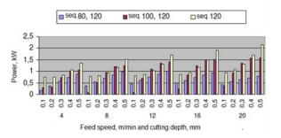
Fig. 3. Variation of power consumption during the perpendicular sanding of black alder wood when using three sanding sequences as a function of feed speed an cutting depth
