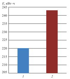
**Fig. 4.** Comparative characteristics of power generation from various sources: *I* — vegetable raw materials; *2* — torrefied vegetable raw materials
