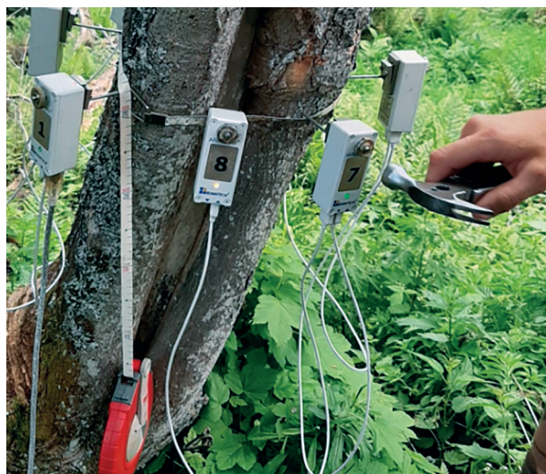
Fig. 2. Location of sensors and induction of sound impulses using a hammer
